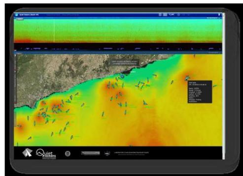
Figure 3 - Screenshot of the dual interface of the real-time passive acoustic monitoring (top) and the real-time noise mapping (bottom)
