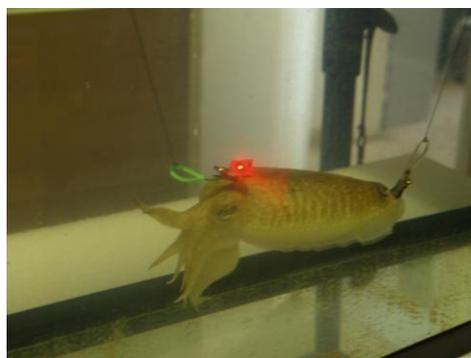
Figure 7 – Laser Doppler Vibrometer technique to determine the onset mechanism of body vibration when a cuttlefish is exposed to sound
